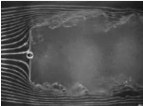
**Figure 3. Wake Flow Behind Flat Plate Body**
