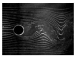
Figure 4. Flow Around Cylinder
