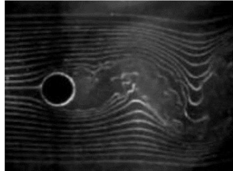
**Figure 4. Flow Around Cylinder**
