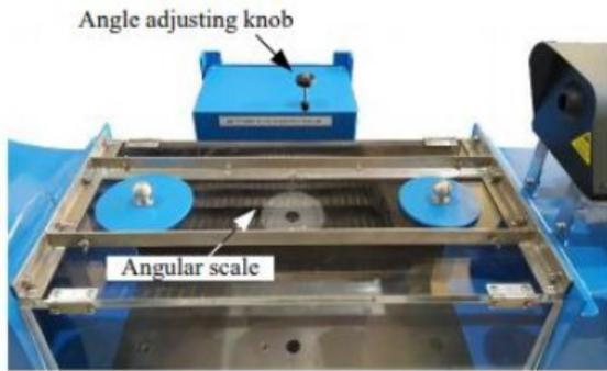
**Figure 6. Scale and Adjusting Knob**
