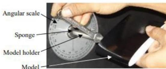
**Figure 8. Model Installation.**
