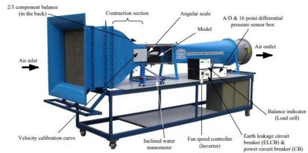
**Figure 10. Subsonic Wind Tunnel**
