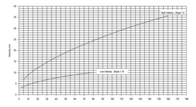
Contraction Section Differential Pressure, mmH<sub>2</sub>O
