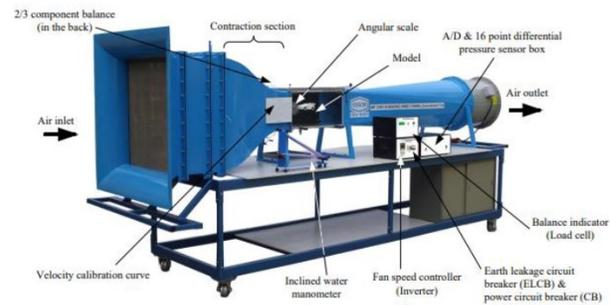
**Figure 10. Subsonic Wind Tunnel**
