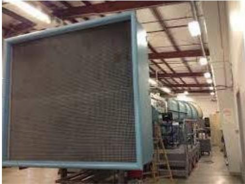
**Figure 12. Wind Tunnel with Acoustic Baffles and Dense Honeycomb**
