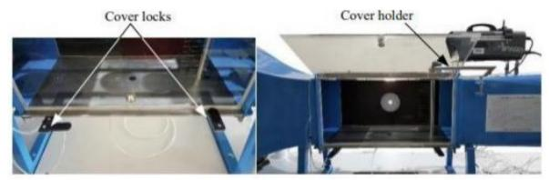
1.2. Open the test section front cover by opening the cover lock as shown in Figure 16.
