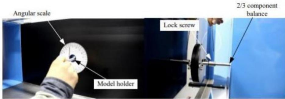
**Figure 17. Install the model holder and set up the scale index**
