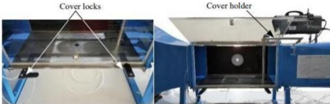
Figure 16. Front view of test section and cover
