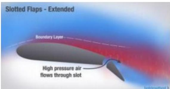
**Fowler Flaps** - Fowler flaps are a type of slotted flap. This flap design not only changes the camber of the wing, it also increases the wing area. The fowler flap rolls
